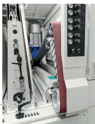
Extractable internal crossbelt unit with 5000 mm belt length.
