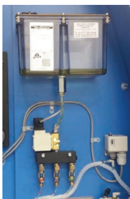
Blade and pulley lubrication
