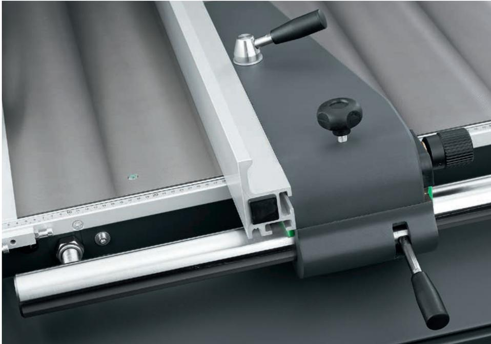
**Rip fence with manual fine adjustment.** Setting the fence is easy; the precision fine adjustment makes for great accuracy. The hard chrome-plated round bar system ensures the fence moves smoothly. The rip fence drops down clear of the machine table level to free up extra space for dividing large panels.
