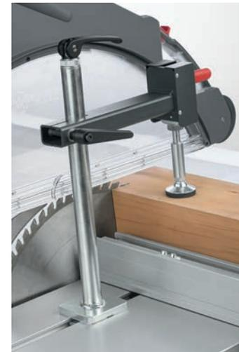
**Manual quick-action clamp.** The alternative to the pneumatic quick-action clamp. The manual quick-action clamp can be easily positioned on the sliding table and fixed. The workpiece is then firmly secured on the table and the crosscut fence. It has a clamping height of up to 200 mm and provides extra safety at very little extra cost. Not available in CE region.
