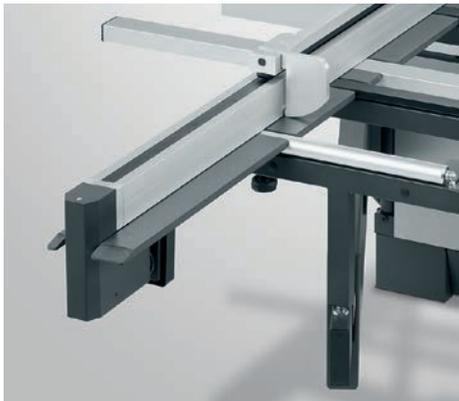
**UNO 90 CNC crosscut fence.** Fixed in the 90° position, the UNO 90 CNC crosscut fence enables efficient and precise execution of right-angled cuts. The flip stop has a maximum travel of 1,900 mm as standard, but the extension supplied can be fitted manually to give a longer fence with a maximum dimension of 2,900 mm if required.
