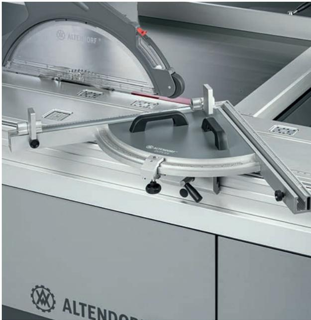
**DUPLEX double-sided mitre fence.** DUPLEX fences enable bevel cuts at any angle between 0 and 90° with speed and precision. Set it to 45° and a mitre cut can be made on both sides of the workpiece without further adjustments. Dimensions of the flip stops are set using a measuring scale and magnifier. All DUPLEX fences can be positioned anywhere along the entire length of the table. With no more than 17 kg all DUPLEX models now have improved handling.
