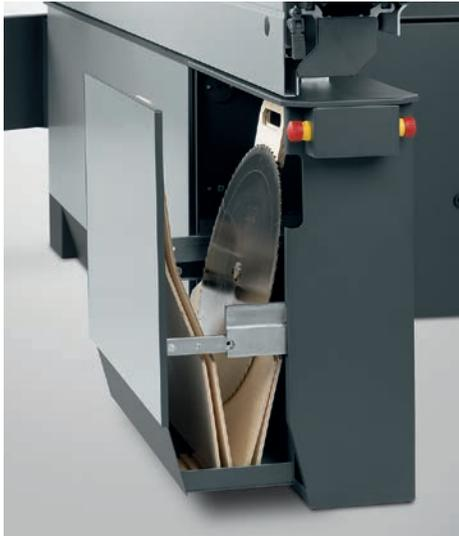
**Toolbox.** The practical toolbox is a drawer capable of holding up to six tool carriers (maximum saw blade diameter 550 mm) ready for use. Four tool carriers are included in the standard scope of supply. This option requires a minimum sliding table length of 3,000 mm.
