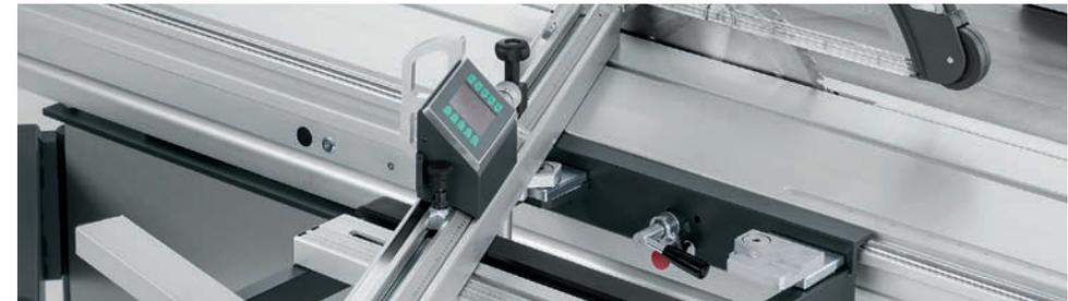
**DIGIT L:** for 1/10 mm accuracy when setting the length dimension. The display shows all stop settings applied. The central measuring and display unit calibrates the entire system in one operation. Two flip stops with fine adjustment, two batteries and a charger are included.
