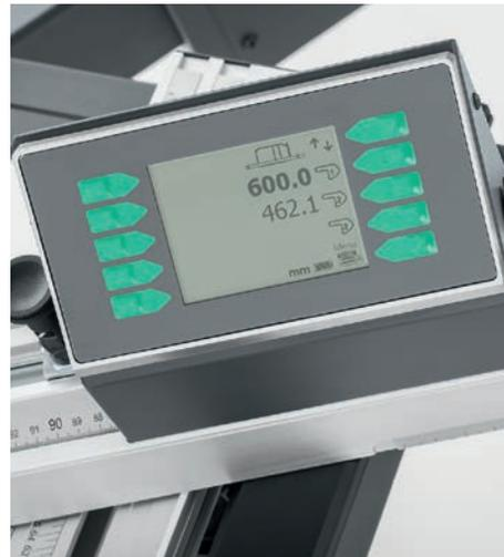
**DIGIT L:** for 1/10 mm accuracy when setting the length dimension. The display shows all stop settings applied. The central measuring and display unit calibrates the entire system in one operation. Two flip stops with fine adjustment, two batteries and a charger are included.
