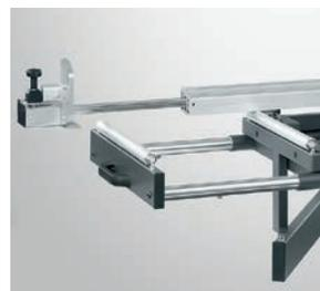
**Pull-out cross slide extension.** This option makes it easier to cut longer/wider workpieces and increases the width of the support area for the manual crosscut fence.
