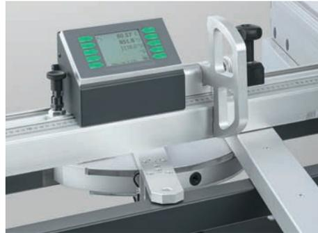
**DIGIT LD:** for 1/10 mm accuracy when setting the length dimension. The display shows all stop settings applied. The central measuring and display unit calibrates the entire system in one operation and angles are displayed in digital format, enabling a level of precision of  $\pm 1/100^\circ$ . The length dimension is calculated automatically as a function of the mitre angle. Two flip stops with fine adjustment, two batteries and a charger are included.
