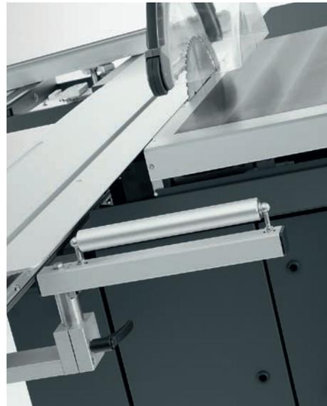
**Front support roller.** The 300 mm-wide front support roller is particularly useful when cutting longer workpieces on the rip fence. It can be folded down through 90° in one movement to stow under the sliding table (minimum length 3,000 mm) when not required.
