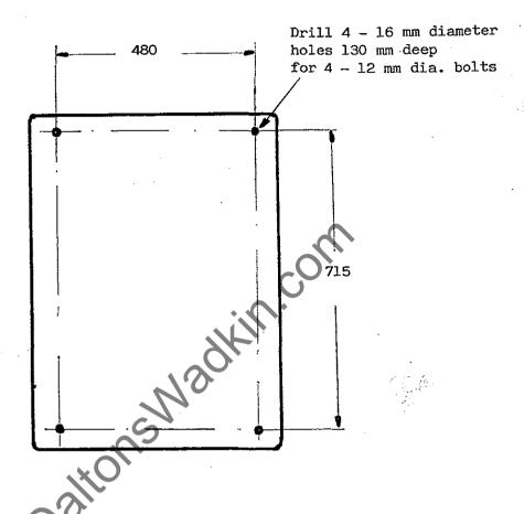
Machine must be positioned and levelled on a solid floor.
