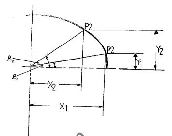
Using  $\frac{1}{2}$  the major axis as the radius, r, we can use the above formulae. When the Y dimension has been calculated we can then multiply this by the following ratio:-
