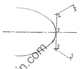
Point 1 is 20 mm away from the edge of the ellipse and 40 mm below Y0. From this point we can move to point 2 putting on cutter compensation. [This distance should be large enough for cutters up to about 27 mm radius].
