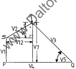
Points P, Q and S are easy to determine in terms of distance from the datum point. Point R, however needs to be calculated.
