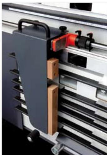
The robust folding measuring stop (with fine adjustment) on a 30 mm steel shaft and square stop-extension is supplied as standard. The need for lifting heavy panels on to the mid fence is no longer necessary.
