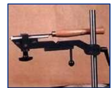
Gouge Tool holder in Inspection Position
