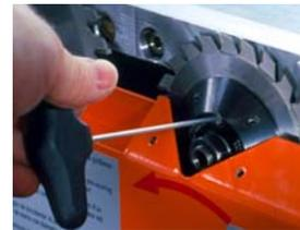
release the clamping screw      turn the spindle
