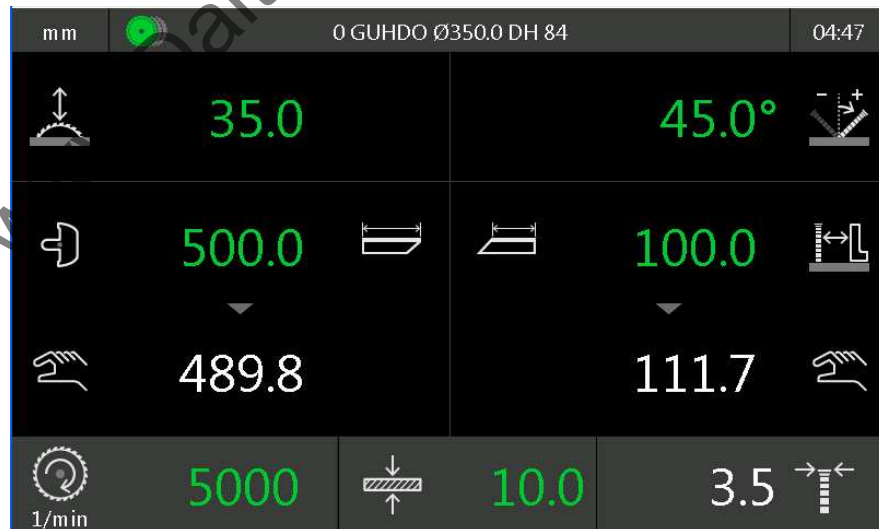
Fig. 6-37 Display of the auxiliary dimensions of the tilted saw blade
