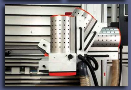
The ADVANCE **clamps** can lift panels up to 150 kgs (up to 225 kgs with 3 clamps). Also several panels can be clamped and lifted simultaneously with a maximum overall material thickness of 55 mm.
