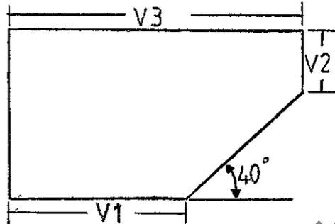
Write a programme for the above component. Again input variables are V1, V2 and V3.
