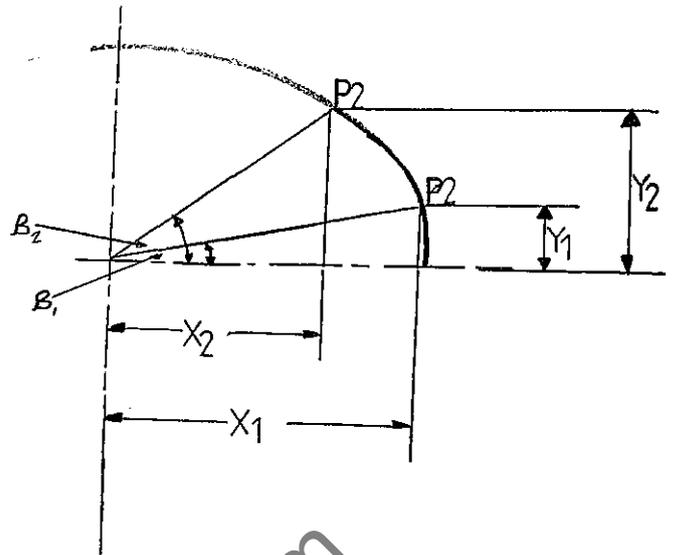
Using  $\frac{1}{2}$  the major axis as the radius,  $r$ , we can use the above formulae. When the Y dimension has been calculated we can then multiply this by the following ratio:-
