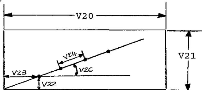
Write a programme to drill a series of holes in a panel. The holes are along a straight line which may rotate through an angle - V26. The programme must halt if faulty data is input ie:- The board not being long enough or wide enough to accept the number of holes or the angle being more than 90°.
