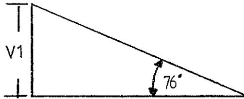
Write a programme to machine this component. Input variable is V1; Angle is always 76 degrees.
