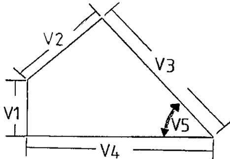
The object, here, is to formulate a programme to machine the above shape of component. Notice, though, that we do not have fixed sizes, we have variables.
