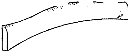
Type of jig required for shaping and moulding curved chair backs, etc.
