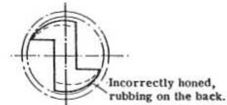
Dotted line indicates necessary grinding to restore cutting edges.
