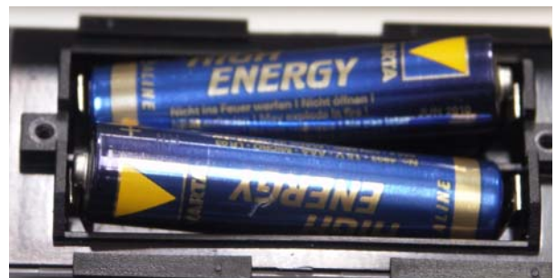
Fig. 7-13: Insert/replace batteries, ensuring correct polarity!
