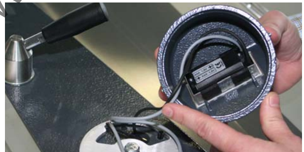
Fig. 7-12: Detach the display housing
