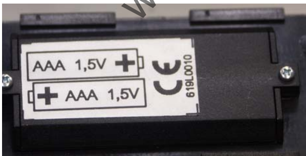
Fig. 7-11: Loosen and withdraw screws and remove cover
