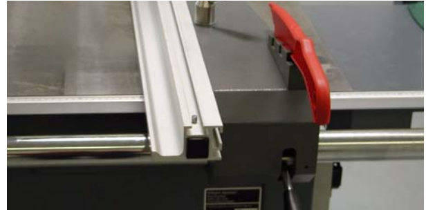
Fig. 3-6: Extension fence height adjustment
