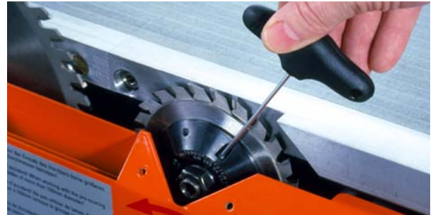
Fig. 7-7: Release the clamping screw
