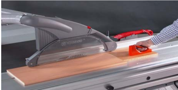
Fig. 3-9: Cutting of strips
