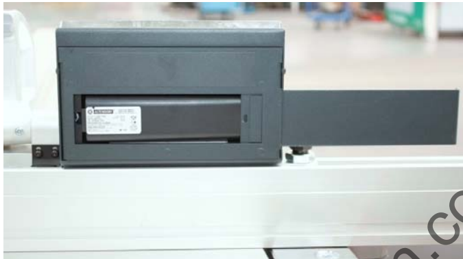
Fig. 6-80 Changing the rechargeable battery for DIGIT L , DIGIT LD
