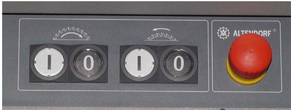
Fig. 6-22 Switches for saw drives
