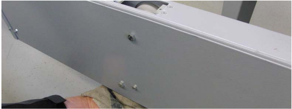
Fig. 7-9 Clean the roller from below
