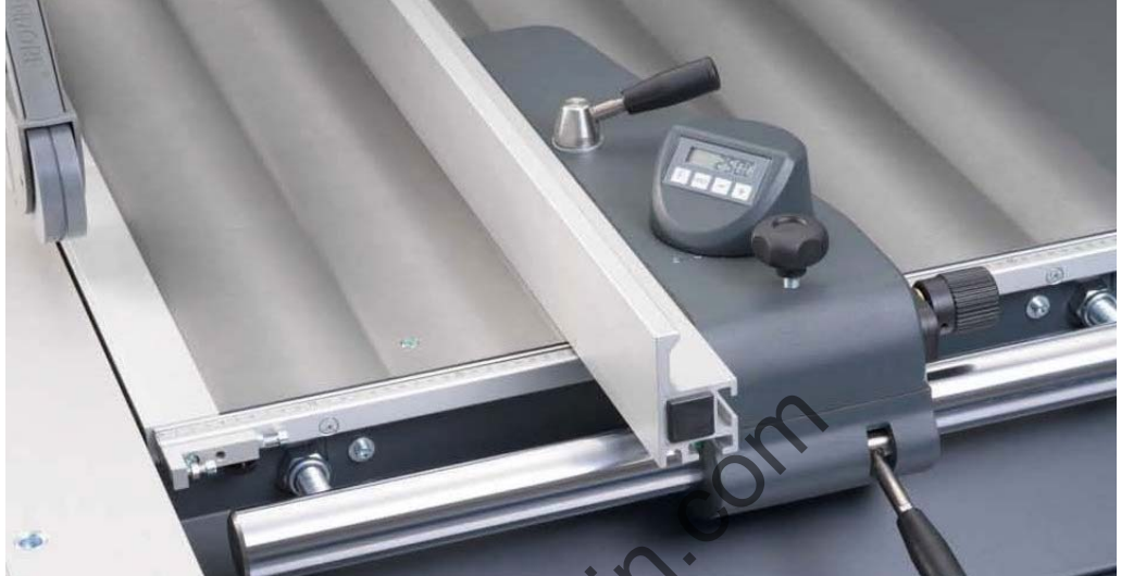
Fig. 6-84 Rip fence with Digit X
