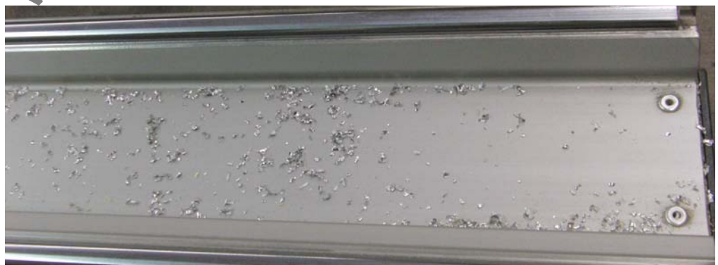
Fig. 7-2 Remove chips from the bottom carriage of the sliding table
