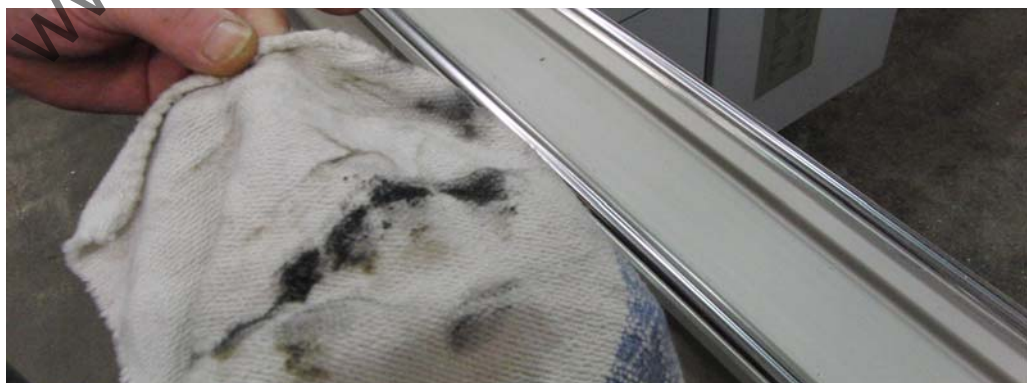
Fig. 7-5 Dirt from the bottom of the sliding table guide
