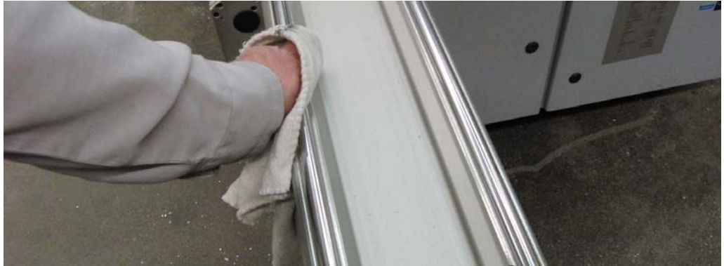
Fig. 7-3 Remove dirt and resin residue from the guide of the sliding table using a cloth soaked in spirit
