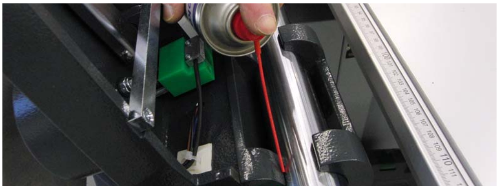
Fig. 7-11 Spray round bar. Subsequently move the block up and down.
