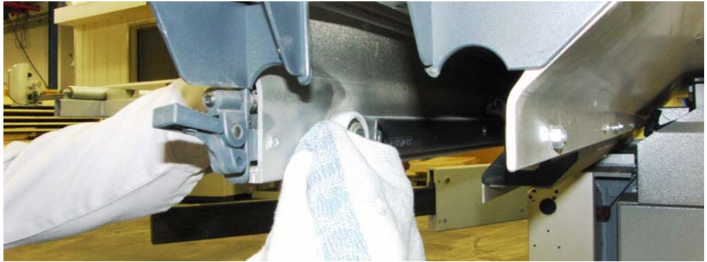
Fig. 7-6 Cleaning of the sub-rollers of the sliding table
